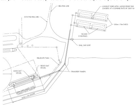
Scope included site visit to finalise port facility requirements including berth location, rail loop, stockyard, conveyors, wharf and shiploader. The port was limited to Panamax vessels so transhipment options were researched so that Cape vessels could be loaded offshore.
