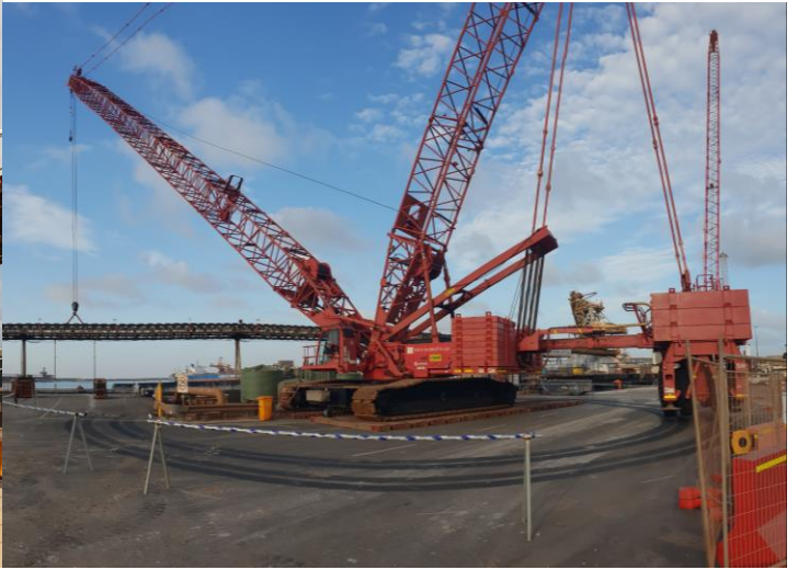
400t crane with 150t maxer at 15m radius
